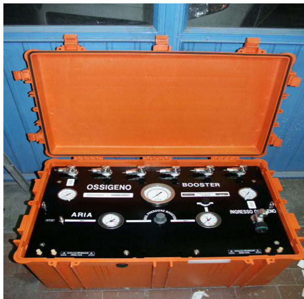
Waterproof case, air drive , 7 cylinder housing, speed regulation
